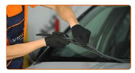
Remove the blade from the wiper arm.
