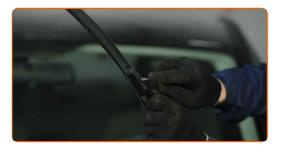
Remove the blade from the wiper arm.
