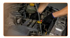
6 Unscrew the ignition coil bracket. Use Torx T40. Use a ratchet wrench.
