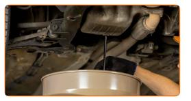
Replacement: engine oil and filter – Opel Corsa C. AUTODOC experts recommend:
