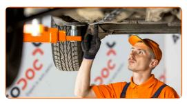
Loosen the filter fastenings. Use a Phillips screwdriver.
