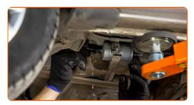
7 Tighten the fuel filter fasteners. Use a Phillips screwdriver.
