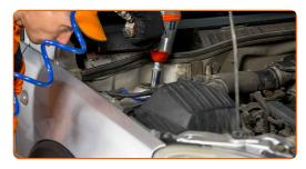
Install the shock strut mount cap.
