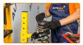
Tighten the shock strut piston rod nut. Use HEX No.H6. Use a combination spanner #19. Use a torque wrench. Tighten it to 55 nm torque.
