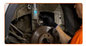
Disconnect the fastener of the ABS sensor cable from the shock absorber strut.
