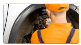
Connect the fastener of the ABS sensor cable to the shock absorber strut.
