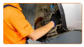
Tighten the lower fasteners connecting the shock strut to the steering knuckle. Use a combination spanner #18. Use a drive socket #18. Use a torque wrench. Tighten it to 80 Nm torque.+75°
