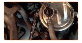
Disconnect the pipe from the fuel filter.
