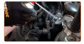
Zerosen the fastening clamp of the fuel filter pipe. Use clic-R collar pliers.
