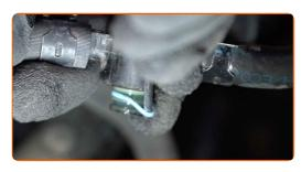
13 Install new o-rings. Use a flat screwdriver.
