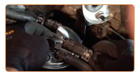
Tighten the fuel filter fasteners. Use a drive socket #10.
