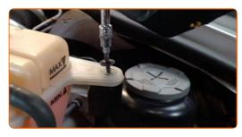
5 Remove the coolant reservoir.
