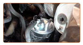
Attach the pipe to the fuel filter.
