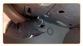
Install the side trim panel. Position the part using the guides and lock the fasteners.
