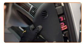
Unscrew the glove box fastening screws. Use a drive socket #8. Use a ratchet wrench.
