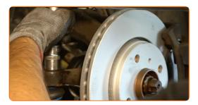
Treat the fastener connecting the tie rod end to the steering knuckle. Use copper grease.
