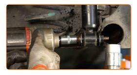
13 Remove the fastening bolt.
