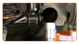
Remove the mounting from under the rear axle beam.
