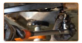
Tighten the ball joint fastener. Use a combination spanner #18. Use a torque wrench. Tighten it to 98 nm torque.
