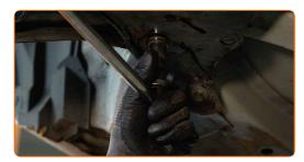
Remove the rear fastener of the control arm. Use a drive socket #17.
