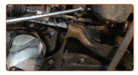
Unscrew the rear fastener connecting the control arm to the subframe. Use a drive socket #17. Use a tap wrench.
