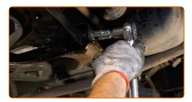
Tighten the rear fastener of the control arm. Use a drive socket #17. Use a torque wrench. Tighten it to 110 Nm torque.
