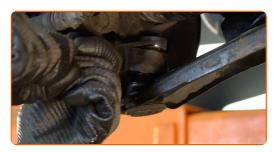
Unscrew the front arm fastener. Use a drive socket #17. Use a tap wrench.
