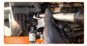
Remove the support from under the arm.
