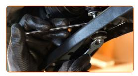
Tighten the fastener connecting the stabilizer bar with the control arm. Use a drive socket #12. Use a torque wrench. Tighten it to 18 Nm torque.
