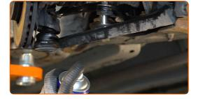
Unscrew the fastener connecting the stabilizer link to the stabilizer bar. Use a combination spanner #12.
