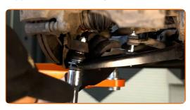
Tighten the fastener connecting the stabilizer bar with the control arm. Use a combination spanner #10. Use a combination spanner #13. Use a drive socket #13. Use a torque wrench. Tighten it to 18 Nm torque.
