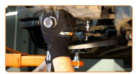
Remove the support from under the arm.
