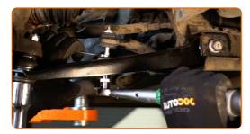
Tighten the fastener connecting the stabilizer link to the stabilizer bar. Use a combination spanner #10. Use a drive socket #13. Use a torque wrench. Tighten it to 18 Nm torque.
