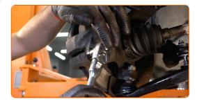
10 Remove the brake caliper.
