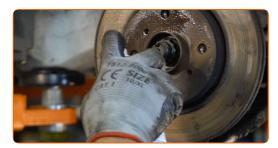
Unscrew the brake disc fastening. Use Torx T30. Use an impact screwdriver.
