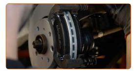
27 Install the brake caliper and fix it. Use a drive socket #13. Use a torque wrench. Tighten it to 30 Nm torque.
