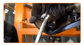
Remove the caliper bracket.
