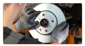
Tighten the brake disc fastening. Use Torx T30. Use a torque wrench. Tighten it to 5 Nm torque.
