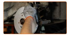
Tighten the brake caliper bracket. Use a drive socket #17. Use a torque wrench. Tighten it to 89 Nm torque.
