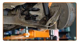
Tighten the lower fastener of the shock absorber. Use a drive socket #E14. Use a torque wrench. Tighten it to 110 Nm torque.
