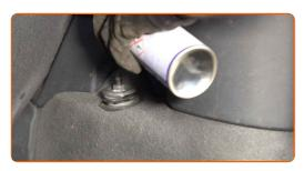
Loosen the upper fastener of the shock absorber. Use a drive socket #16. Use a shock absorber socket DDNº6. Use a ratchet wrench.
