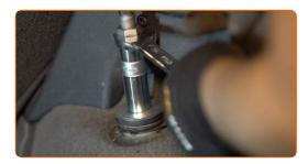
Treat the shock absorber fasteners. Use copper grease.
