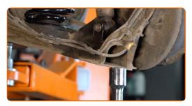
Unscrew the lower fastener of the shock absorber. Use a drive socket #E14.
