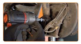
14 Remove the fastening bolt.
