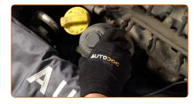
Screw in the fasteners of the protective case of the oil filter housing. Use a drive socket #10. Use a ratchet wrench.
