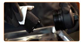
Remove the oil filter cover O-ring. Use a flat screwdriver.
