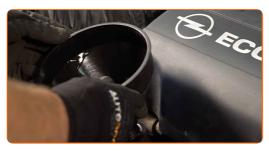
Pour oil into the engine through the filler. Required amount of oil: 3.2 l.
