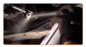
Screw in the new drainage plug and tighten it. Use Torx T40. Use a torque wrench. Tighten it to 20 Nm torque.
