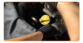
Screw in the fasteners of the protective case of the oil filter housing. Use Torx T30.
