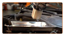
Detach the old filter cartridge from the filter housing cover.
