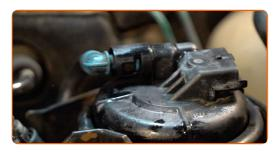
Attach the fuel pressure sensor connector.
