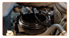
13 Install the new sealing ring.
