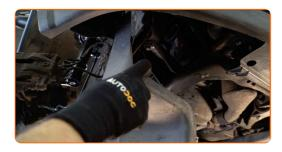
Pull aside the V-ribbed belt tensioner pulley. Use a combination spanner #15.
