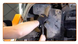
Install and tighten the wheel arch cover fasteners. Use Torx T20.
