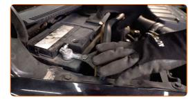
Screw in the fastener of the wiper cowl grille located on the left side. Use Torx T25.
