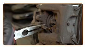
Clean the fasteners of the brake pad wear sensor wiring harness. Use a wire brush. Use WD-40 spray.
