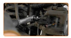
Treat the brake pad wear sensor plug. Use dielectric grease.
