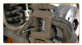
Tighten the brake caliper fasteners. Use HEX No.H7. Use a torque wrench. Tighten it to 25 Nm torque.
