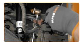
Unscrew the fasteners of the brake pad wear sensor wiring harness. Use Torx E10. Use a ratchet wrench.
