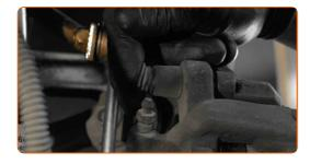
Attach the brake pad wear sensor wiring harness.
