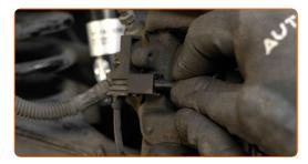
Install the brake caliper retaining spring.
