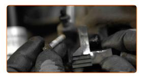
Detach the brake pad wear sensor wiring harness.
