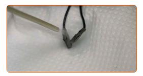
9 Attach the mirror heating connectors.
