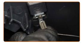
Fit the mirror glass into position. Make sure you hear a click indicating that it is locked in place.
