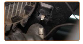
Unscrew the mirror cover frame fasteners. Use Torx T10.
