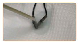
27 Attach the mirror heating connectors.
