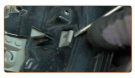
Remove the turn signal repeater light.
