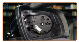
Snap the mirror cover frame tabs back into place. Make sure you hear a click indicating that it is locked in place.
