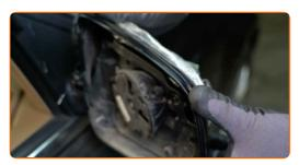
Snap the tabs of the turn signal repeater light back on the mirror cover. Make sure you hear a click indicating that it is locked in place.
