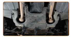
Tighten the fasteners of the oil pan lower cover. Use a drive socket #8. Use a ratchet wrench.
