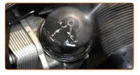
Unscrew the filter housing cap together with the old filter element. Use the 74/15F socket. Use a ratchet wrench.
