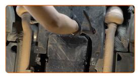
Put a waste oil container with at least 9 l capacity under the drainage hole.
