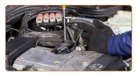
7 Detach the vacuum pipe. Use a flat screwdriver.
