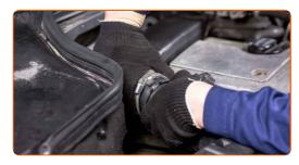
Unscrew the clamp that fastens the air filter hose to the throttle body. Use a flat screwdriver.
