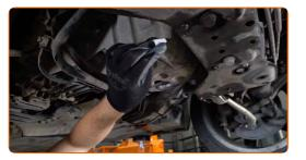
Screw in the new drainage plug and tighten it. Use a drive socket #24. Use a torque wrench. Tighten it to 30 Nm torque.
