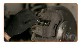
Tighten the brake caliper fasteners. Use a combination spanner #15. Use a drive socket #13. Use a torque wrench. Tighten it to 30 Nm torque.
