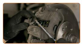
Remove the brake caliper.
