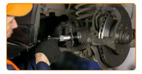
Install the brake caliper and fix it.
