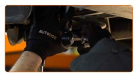
Screw in the lower fastener of the shock absorber. Use a drive socket #19.
