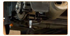
Tighten the lower fastener of the shock absorber. Use a drive socket #19. Use a torque wrench. Tighten it to 110 Nm torque.
