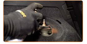
Install the mount cap on the shock absorber upper fastener.
