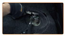
Remove the fastening bolt. Use a drive socket #19.
