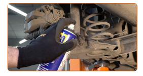
Unscrew the lower fastener of the shock absorber. Use a drive socket #19. Use a tap wrench.
