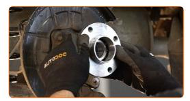
Tighten the hub. Use a drive socket #32. Use a torque wrench. Tighten it to 224 Nm torque.
