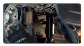
Remove the caliper bracket.
