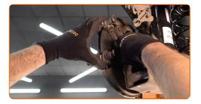
Tighten the brake caliper bracket. Use a drive socket #17. Use a torque wrench. Tighten it to 62 Nm torque.
