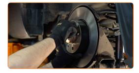
Tighten the brake disc fastening. Use a drive socket #12. Use a torque wrench. Tighten it to 10 Nm torque.
