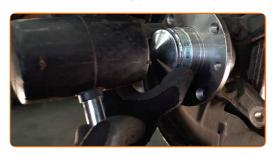
Treat the hub where it contacts the brake disk. Use copper grease.
