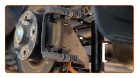
Unscrew the caliper bracket fastening. Use a drive socket #17. Use a tap wrench.
