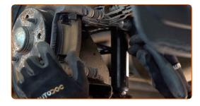
Remove the caliper bracket.
