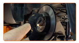
Tighten the brake disc fastening. Use a drive socket #12. Use a torque wrench. Tighten it to 10 Nm torque.
