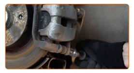
Remove the brake caliper. Use a crowbar.
