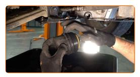
Screw the new filter into its place.
