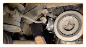
Install a new oil filter housing cover and tighten it. Use the 76/14-F socket. Use a torque wrench. Tighten it to 25 Nm torque.
