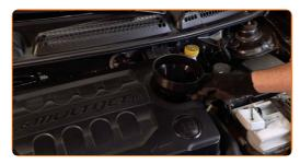
Pour oil into the engine through the filler. Required amount of oil: 4.6 l.
