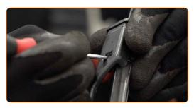
Remove the blade from the wiper arm.
