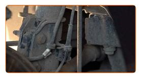
Clean the fasteners connecting the stabiliser link to the shock strut, and those connecting the shock strut to the steering knuckle.
