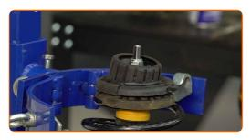
Remove the assembled shock strut.
