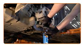
Unscrew the lower fastener connecting the shock strut to the steering knuckle. Use a combination spanner #15. Use a drive socket #17. Use a tap wrench.
