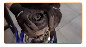
Release the coil spring.
