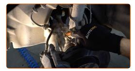
Unscrew the nut and remove the stabilizer rod from the shock strut. Use a combination spanner #17. Use a ratchet wrench.
