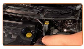
Loosen the upper fastener of the shock strut mount. Use a combination spanner #19.
