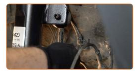
Tighten the fastener connecting the stabilizer link to the shock strut. Use a combination spanner #17. Use a torque wrench. Tighten it to 55 Nm torque.
