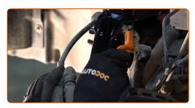
Fix the shock absorber strut on the steering knuckle.
