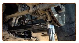
Tighten the ball joint fastener. Use a drive socket #17. Use a combination spanner #17. Use a torque wrench. Tighten it to 65 nm torque.
