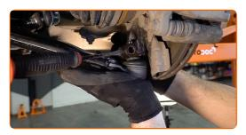
20 Install the control arm fasteners.
