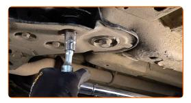
Remove the support from under the arm.
