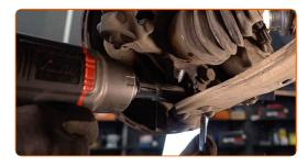
10 Remove the fastening bolt.
