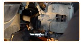
11 Remove the brake caliper.
