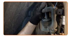
Install the brake caliper and fix it. Use a drive socket #13. Use a torque wrench. Tighten it to 30 Nm torque.
