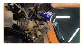
Unscrew the caliper bracket fastening. Use a drive socket #19. Use a ratchet wrench. Use a tap wrench.
