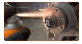
20 Install the brake disc.
