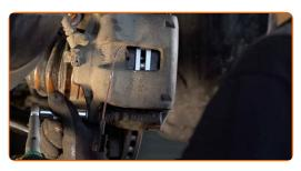
Connect the brake pad wear sensor plug.
