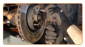
18 Remove the brake disc.
