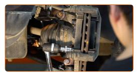
Remove the caliper bracket.
