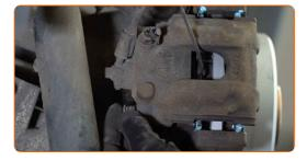
Install the brake caliper retaining spring.
