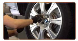
Lower the car and working in a cross order, tighten the wheel bolts. Use a torque wrench. Tighten it to 140 nm torque.
