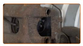
14 Remove the brake caliper.
