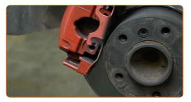
18 Remove the brake caliper.
