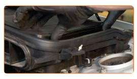
Install the air duct housing.
