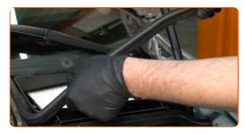
Remove the cabin air filter housing.
