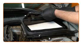
Remove the cabin filter housing seal.
