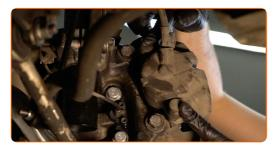
27 Install the brake caliper retaining spring.
