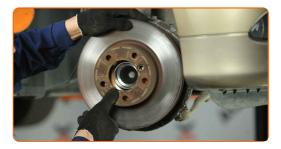
Tighten the brake disc fastening. Use HEX No.H6. Use a torque wrench. Tighten it to 16 Nm torque.
