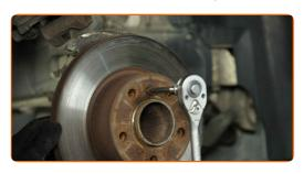
Remove the brake disc.
