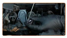
Take out the ignition coil from the spark plug well.
