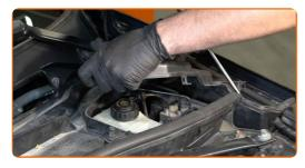
6 Detach the connectors from the climate control sensors.
