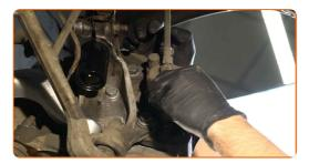
Install the brake caliper retaining spring.
