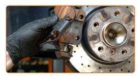
Remove the brake caliper.
