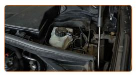
Unscrew the brake fluid reservoir cap.
