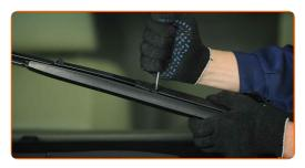
Remove the blade from the wiper arm.
