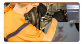
Disconnect the tie rod end from the steering knuckle. Use a ball joint puller. Use a hammer.
