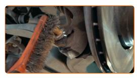
Remove the fastening bolt. Use a drive socket #18. Use a crowbar.
