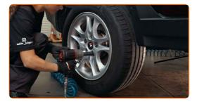
Lower the car and working in a cross order, tighten the wheel bolts. Use wheel impact socket #17. Use a torque wrench. Tighten it to 140 Nm torque.
