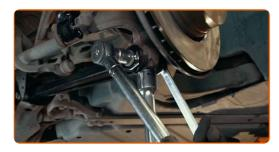
Tighten the fastener connecting the control arm to the subframe. Use a drive socket #18. Use a torque wrench. Tighten it to 77 Nm torque.
