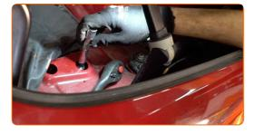
Tighten the lower fastener of the shock absorber. Use a drive socket #18. Use a torque wrench. Tighten it to 100 Nm torque.
