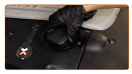
Tighten the oil filler cap.
