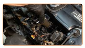
Plug in the ignition coil connector.
