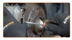
Remove the brake caliper.
