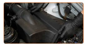
Remove the air filter housing.
