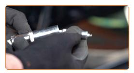
Screw new spark plugs and tighten them. Use the spark plug socket #16. Use a torque wrench. Tighten it to 27 nm torque.
