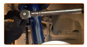
Tighten the fastener connecting the stabilizer link to the stabilizer bar. Use a drive socket #17. Use a combination spanner #17. Use a torque wrench. Tighten it to 55 Nm torque.
