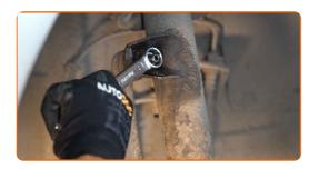
Unscrew the fastener connecting the stabilizer link to the stabilizer bar. Use HEX No.H7. Use a combination spanner #17. Use a ratchet wrench.
