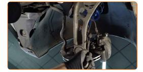
Install a new rod, tighten the fasteners.
