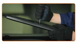
Remove the blade from the wiper arm.
